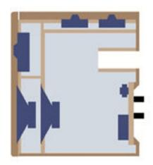
A sealed sub-volume contains the main HF drive unit a modified SEAS XL SONOMEX domed XL unit with additional damping and support.
