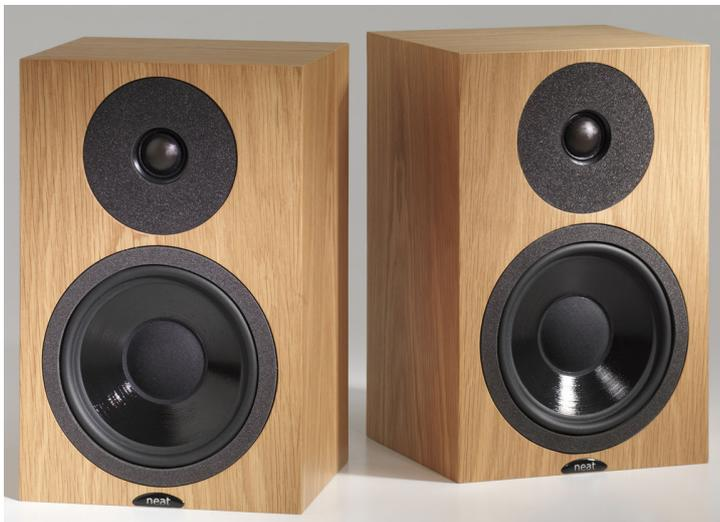
The main drive unit is the latest version of that used in the upmarket **Ultimatum** range; a 6.5" doped paper cone with a ferrite magnet assembly and vented voice coil to enable high power handling without compression.
