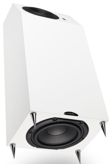
Visually deceptive, the Iota Alpha required some unorthodox engineering. The basis of the original Iota (the main drive unit and the EMIT type planar magnetic tweeter) is housed in the top section of the cabinet, in a sealed volume, angled upwards. This section is configured as a two-way closed box loudspeaker. The whole of the ported lower section is dedicated to augmenting the lower frequencies, via a downward-firing 134mm drive unit mounted on the bottom panel.
